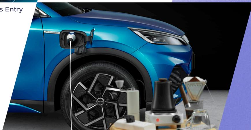
V2L (Vehicle to Load) function can connect 220V power from the car to supply other electrical devices.
